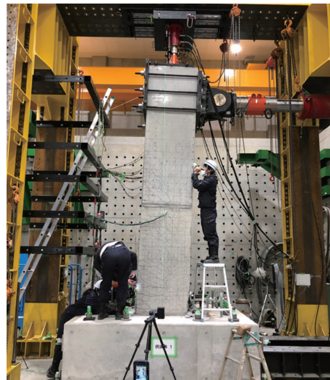
Cyclic loading test of a large RC column specimen
